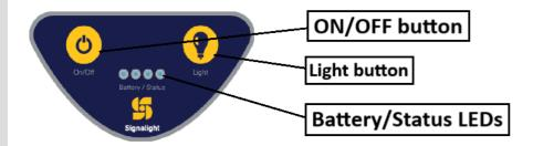
After mechanical installation is done, push the ON/OFF button. This will connect the battery and the POLARIS unit will be powered. As long as the unit is powered the yellow LED from the SIGNALIGHT LOGO will flash every 5 secons. In this moment the lights are in STANDBY mode.
