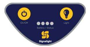
After installation, pressing the On/Off button closes the power circuit between the battery and the lamp.
