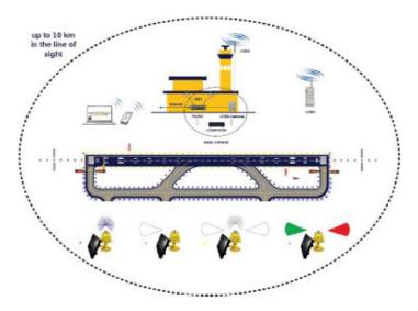
From the POLARIS application the control is more complex. The lights can be controlled individual, in groups, on scenarious and the user can see all the parameters of the lights.
