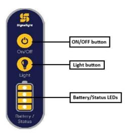
After mechanical installation is done, push the ON/OFF button. This will connect the battery and the POLARIS unit will be powered. As long as the unit is powered the yellow LED from the SIGNALIGHT LOGO will flash every 5 secons. In this moment the lights are in STANDBY mode.
